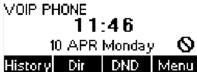
Figure 56 - DND Enabled on All Lines
